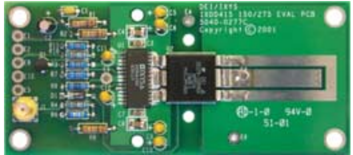
Figure 1 - EVDD415 Evaluation Board DEI DE275-102N06A Device Installed In Low-Power Configuration For Illustration Purposes Only
